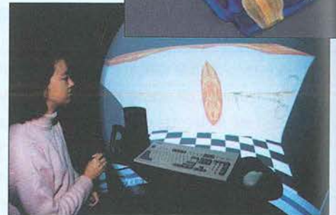
Figure 2 - Simulators with stereoscopy and re-feeding of forces for training surgical procedures [Machado 2001a,b]
