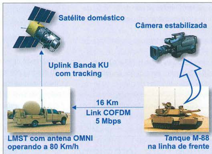
Land Mobile Stabilized Transmitter
