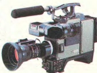
HL-55A, 3/8" 3-Chip FIT CCD • RES: 700 TVL • SENS: f8.0 2000 Lux, SNR 62dB • 400,000 Pixels • CCU: Triax or Multicore • Accepts Beta or MII VCRs
