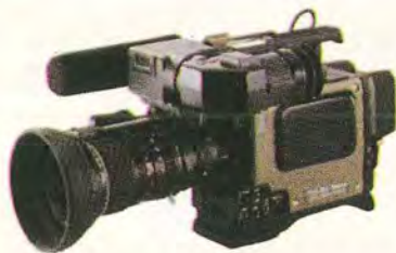
HC 240 1/2" 3-Chip FIT CCD • RES 700 TVL • SENS: f5.6, 2000 Lux, SNR 60dB • 400,000 Pixels • RS-232C Port • Multi-Speed Electronic Shutter • Accepts S-VHS, Beta SP, MII & Hi-8.
