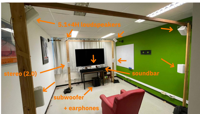
Fig. 6: Auditory test room and sound systems used in the tests.
