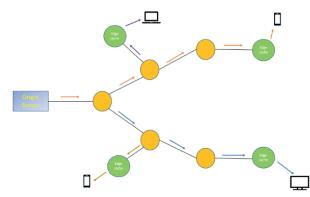
Fig. 8: Example of CDN architecture, with Origin server in blue, nodes in yellow and edge caches in green.
