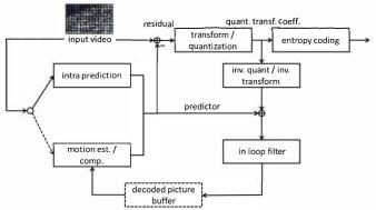
Fig. 1. The block-based hybrid video coding scheme.
