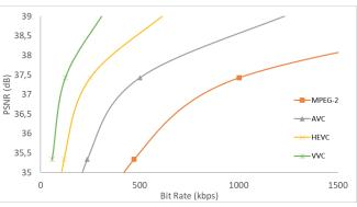
Fig. 2. Video codecs rate distortion performance progression example.
