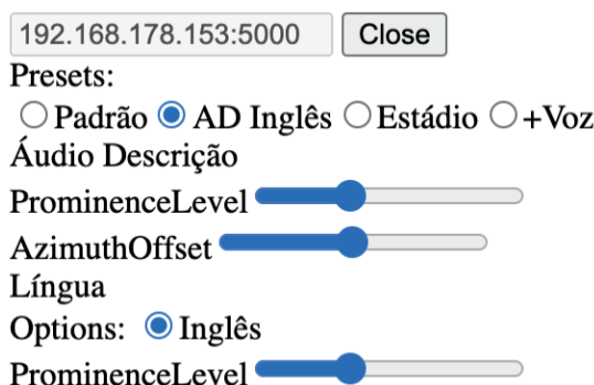
Fig. 4. Illustrates the prototype UI while decoding an audio item with 4 presets. The “ProminenceLevel” slider can be used to control the balance between the corresponding audio switch group or audio object in relation to the overall audio scene.
